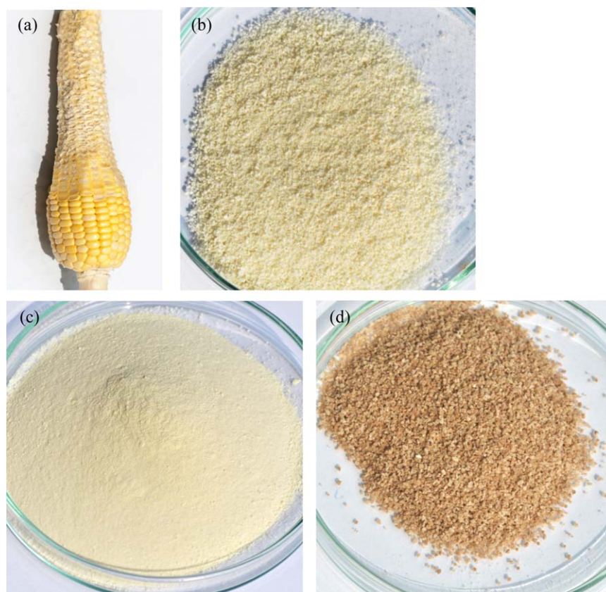
Figure 1. Physical appearance of the (a) corn cob, (b) corn-cob cellulose, (c) PAN-grafted corn-cob cellulose, and (d) polyamidoxime ligand. [Color figure can be viewed in the online issue, which is available at wileyonlinelibrary.com .]
